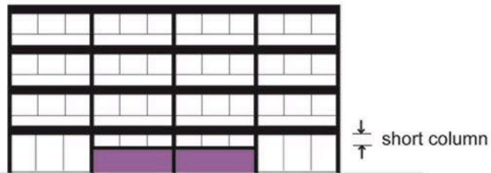
partial floor-height panel infill
